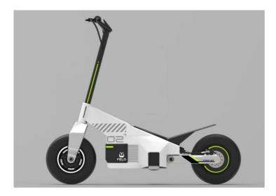
**ADV** 35kw, 400km range, 160km/h speed, 30min full charged by Charging pile (dc charging), touch screen, navigation and other intelligent configuration, V2EX function to provide 20 KWH power for accessories appliances (2024 EDD)
